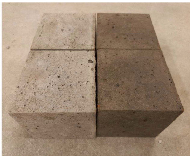
Figure 13. Colour change of PCM-3DPC cubes.
