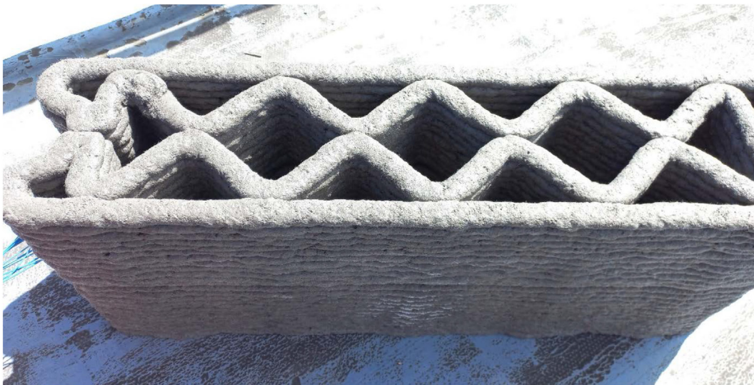
Figure 10. PCM-3DPC facade section used in thermal tests.
