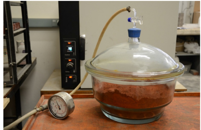
Figure 2. Setup of vacuum desiccator for aggregate impregnation.
