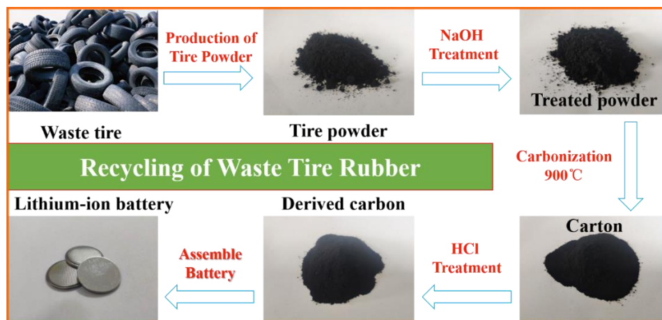
Scheme 1. Schematic preparation procedure for waste tire carbon from waste tires.
