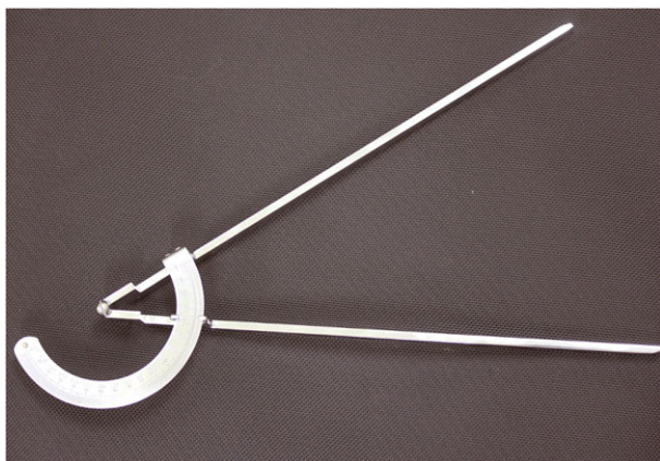
FIGURE 1 Instrument used for measurement. A University of Tokyo-style angle gauge (1° increments, Yasuda Ltd. Tokyo, Japan).
