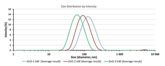
Figure 4. Size distributions of ZnO particles/aggregates obtained by DLS method.
