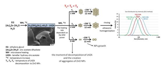
Figure 9. Indicative illustration of formation of ZnO NPs aggregates during the MSS.
