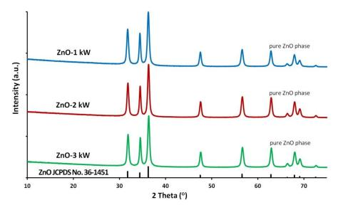
Figure 2. X-ray diffraction patterns of ZnO NPs.
