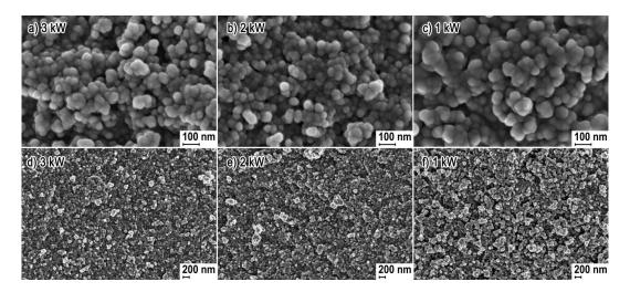
**Figure 1.** SEM images of products of synthesis of ZnO NPs obtained with the microwave radiation power: (**a**,**d**) ZnO-3 kW; (**b**,**e**) ZnO-2 kW; (**c**,**f**) ZnO-1 kW.
