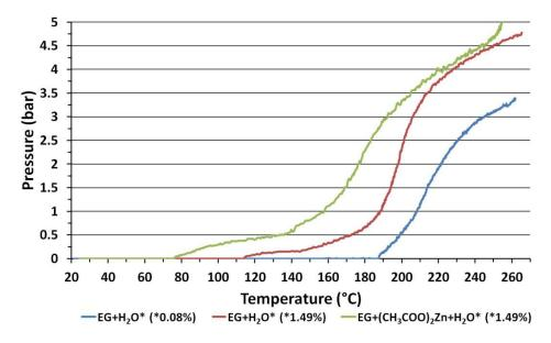
**Figure 6.** Chart presenting the relation between pressure and temperature for: EG with 0.08 wt. % of H<sub>2</sub>O, EG with 1.49 wt. % of H<sub>2</sub>O and precursor  $(Ac)_2Zn \cdot 2H_2O$  dissolved in EG with 1.49 wt. % of H<sub>2</sub>O. Experimental data obtained in the MSS2 microwave reactor.
