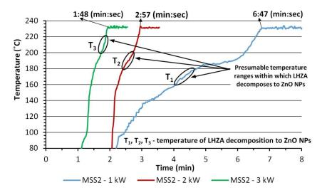
**Figure 8.** Summary of temperature growth profiles for ZnO NPs synthesis in the MSS2 reactor. Source: own data calculated based on the T = f(P) correlation, where: T—temperature, P—pressure in the reactor, f(P)—sixth-order polynomial function.
