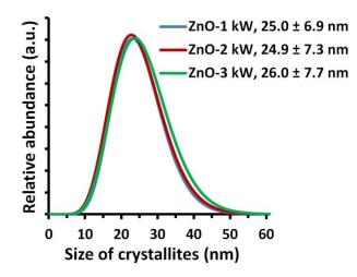
**Figure 3.** Crystallite size distributions of ZnO NPs obtained using Nanopowder XRD Processor Demo, pre  $\alpha$  ver.0.0.8, © Pielaszek Research [66].
