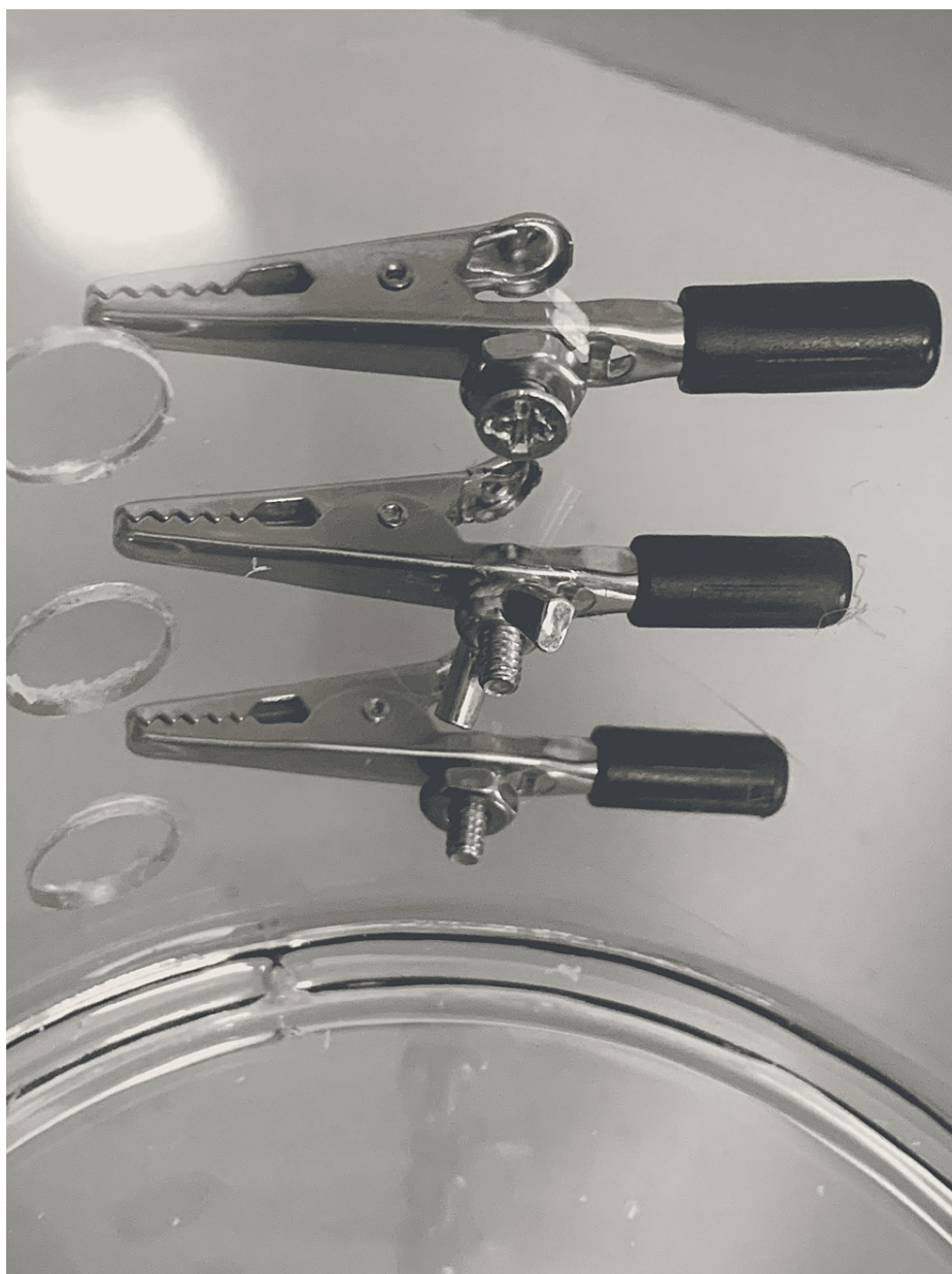
FIGURE 9: Attach alligator clips to the cylinder using nuts and bolts.
