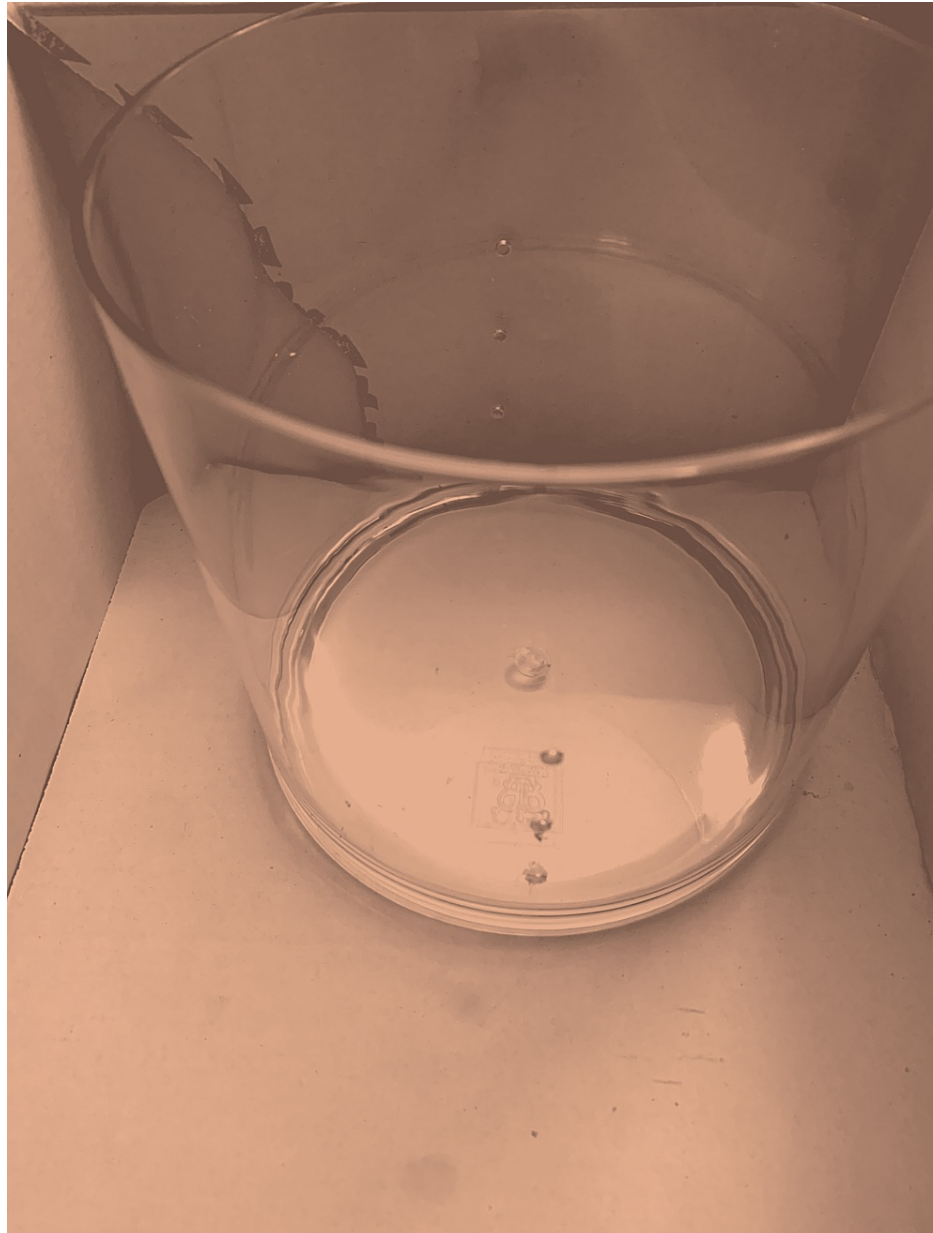
FIGURE 6: Drill initial holes.
