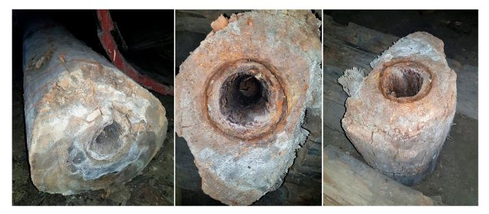
Figure 2. Degraded wooden elements of water pipes found during excavations at Bóżnicza street in Poznań, Poland.
