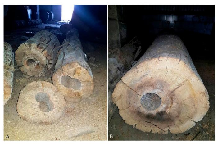
**Figure 1.** Elements of wooden water main excavated at Bóżnicza street in Poznań, Poland: (**A**) more degraded wooden pipes with deep cracks visible in the outer layers; (**B**) an example of a better-preserved log.
