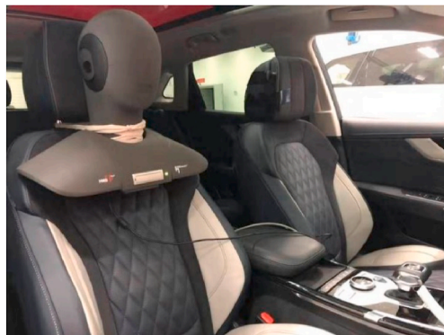
Fig. 2. Measuring point of the in-vehicle sound of the HEAD Acoustics foreman.
