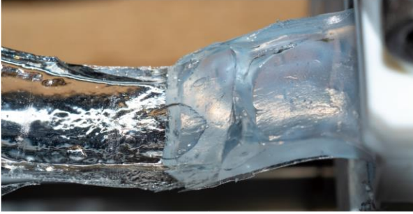
Supplementary Fig. 8. a Photographs of the adhesion test between PDMS BBEs (MM:CL = 1200:1) and Ecoflex. b Curves for shear strength versus displacement of PDMS BBEs (MM:CL = 1200:1) adhered on different substrates.
