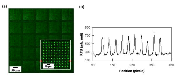
**Figure 4.** Printing and arraying of presynthesized transcribed RNA molecules. (**a**) Microscopy image of the printed pattern of full-length messenger RNA with 5- $\mu$ m array features using the  $\mu$ IP approach; (**b**) Fluorescence distribution plot for a single row of patterned messenger RNA (indicated by the red arrow in (**a**)). RFU, relative fluorescence units.
