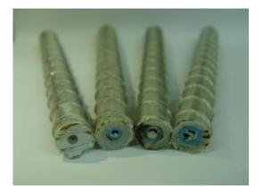
Figure 7. Cross-section of hollow GFRP rebars (D16).
