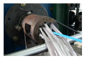
Figure 6. Tube insertion for hollow section.
