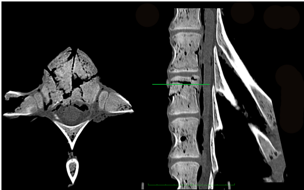
Figure 2 CT scans showing example of the produced incomplete burst fracture in calf spine samples.
