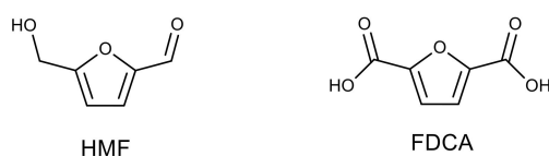
Figure 19. The structures of 2,5-furandicarboxylic acid (FDCA) and 5-hydroxymethylfurfural (HMF).
