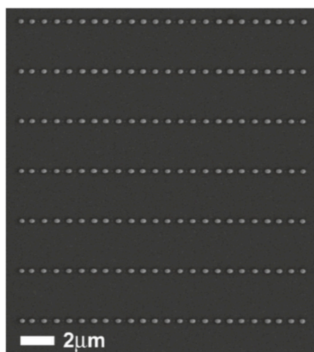
Figure 26. The array of Ni nanoparticles (on Si substrate) arranged in seven lines and obtained by pulsed laser irradiations (wavelength of 248 nm, pulse duration of 18 ns, fluence of 400 mJ/cm 2 , five pulses) of seven nanoscale-thick Ni patterned on the substrate by electron beam lithography. Reproduced with permission from [43]. Copyright American Chemical Society, 2011.
