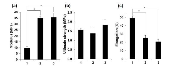
**Figure 4.** Quantitative comparison of the tensile characteristics of non-treated (1), PEG-treated (2) and genipin-crosslinked PEG-treated (3) fibroin membranes. (a) Young's modulus; (b) Ultimate tensile strength; (c) Elongation at break. Bars represents mean  $\pm$  standard error of the mean (n = 6). An asterisk indicates that the difference is statistically significant (p < 0.05).
