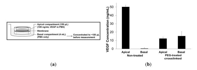
**Figure 5.** Relative permeability of BMSF membranes to VEGF. (a) Schematic representation of the permeability experimental setup. (b) Comparison of VEGF concentrations after 24 h in the apical and basal compartments delimiting the membranes.
