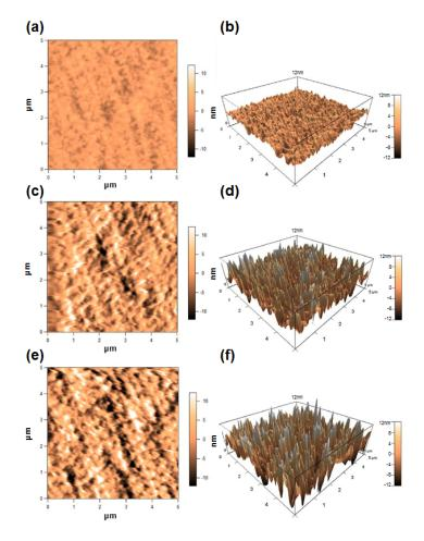
**Figure 2.** 2-D and 3-D AFM images of the surfaces of non-treated (a,b), PEG-treated (c,d) and genipin-crosslinked PEG-treated (e,f) fibroin membranes. Analysed area: 5  $\mu$ m × 5  $\mu$ m.
