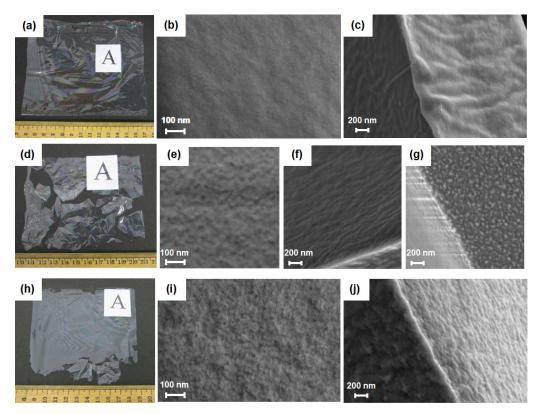
**Figure 1.** Scanning electron micrographs of the *B. mori* silk fibroin (BMSF) membranes. Physical appearance of non-treated (**a**–**c**), PEG-treated (**d**–**g**), and genipin-crosslinked PEG-treated (**h**–**j**) fibroin membranes. (**a**,**d**,**h**) Gross appearance of dried membranes after removal from the casting plate. Images of surfaces (**b**,**e**,**i**), cross-sections (**c**,**f**,**j**) and the edge of the PEG-treated membrane (**g**).
