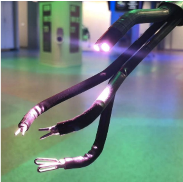
Fig. 2 Multijointed endowristed instrument and scope
