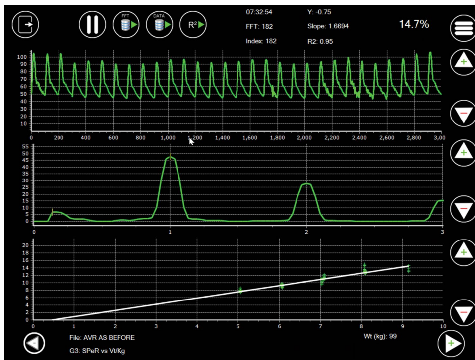
Fig. 1 The application’s user interface. The upper display shows the current sample range of the arterial pressure waveform [Y = pressure (mmHg); X = sample number]. The central display shows the most recently performed spectral analysis [Y = amplitude density; X = frequency (Hz)]. The respiratory and cardiac peaks and the second and third cardiac harmonics are clearly seen. The respiratory peak corresponds to a ventilator rate of 10 bpm and the cardiac peak to
