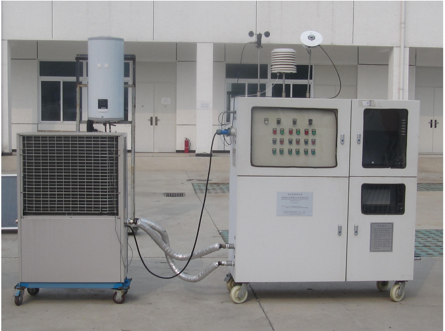
Fig 1. Picture of the detection device used to measure the heat collection rate and heat loss coefficient.
