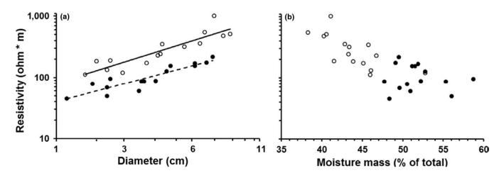
FIGURE 7 Resistivity across a range of diameter (a) and moisture content (b) for the same individuals of Alseis blackiana (solid line and open circles) and Arrabidaea patellifera (dashed line and filled circles). The x-axis is cube-root transformed in panel a
