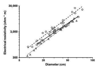
FIGURE 6 Electrical resistivity versus diameter for tree stems >10 cm in diameter (Alseis blackiana = circles, dashed line; Dipteryx panamensis = squares, solid line; and Jacaranda copaia = triangles. dotted line). The x-axis is cube-root transformed
