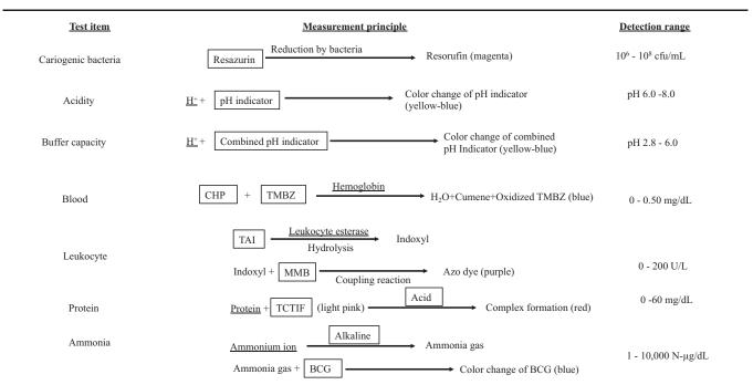
Figure 1. Detection principle of the Salivary Multi Test. \_: Detected substance [: Ingredient in test strip. CHP: cumene hydroperoxide, TMBZ: 3,3',5,5'-tetramethylbenzidine, TAI: 3-(V-toluenesulfonyl-L-alanyloxy)indole, MMB: 2-methoxy-4-(N-morpholino)benzenediazonium, TCTIF: 4,5,6,7-tetrachloro-2',4',5',7'-tetraiodofluorescein disodium salt, BCG: bromocresol green, cfu: colony forming unit.
