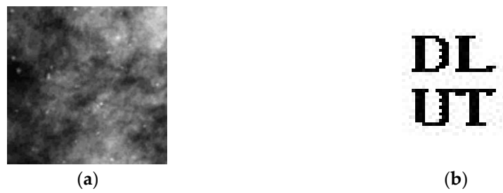
Figure 7. (a) Gaussian noise attack PSNR = 22.4612; (b) recovered logo image from (a) (NC = 0.9824).
