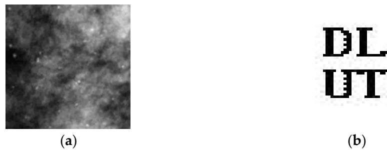
Figure 12. (a) Clipping attack PSNR = 15.7723; (b) recovered logo image from (a) (NC = 0.9688).
