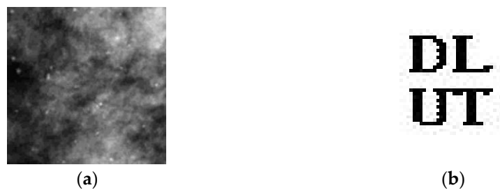
Figure 10. (a) Sharpening attack PSNR = 30.6776; (b) recovered logo image from (a) (NC = 0.9990).
