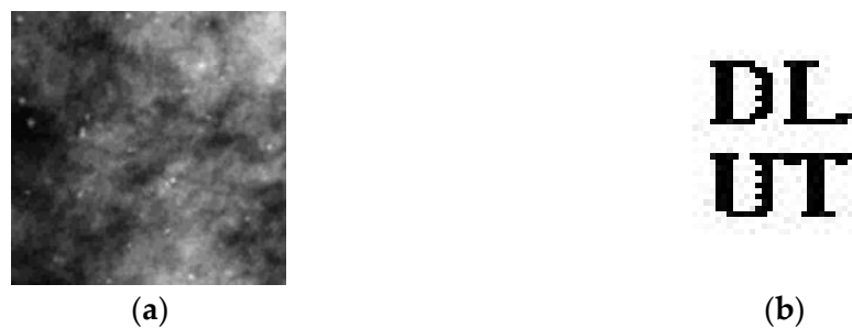
Figure 14. (a) Contrast enhancement attack PSNR = 21.5881; (b) recovered logo image from (a) (NC = 0.9766).
