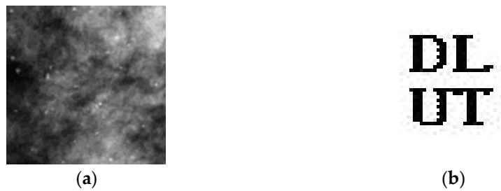
Figure 8. (a) Rotation attack PSNR = 34.7317; (b) recovered logo image from (a) (NC = 1).
