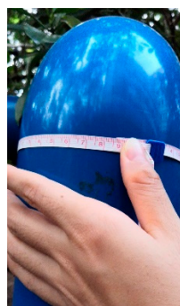
Figure 10. Manual measurement with tape for the circumference (outer diameter) of a joint section.
