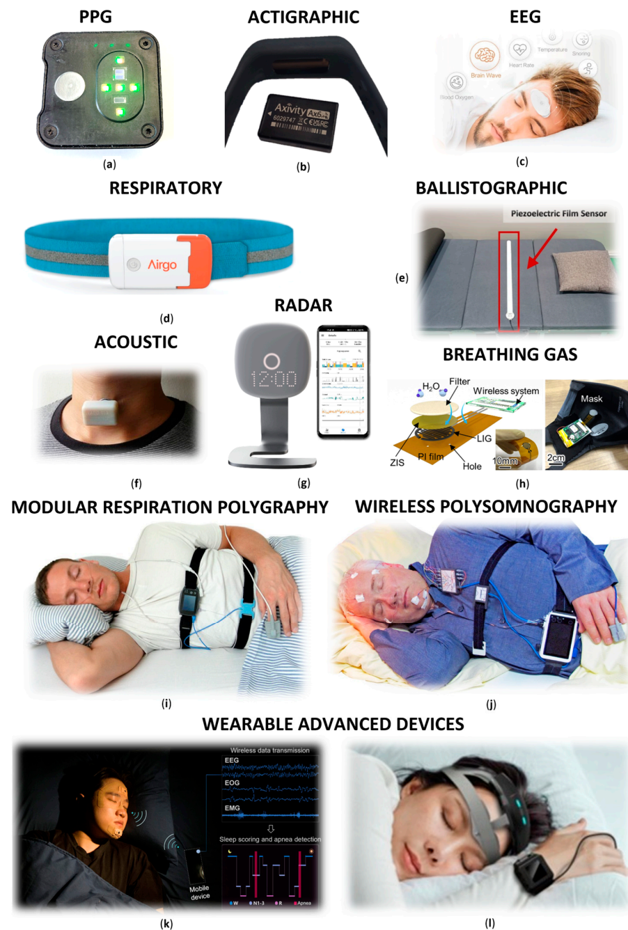
Figure 2. Interesting examples of the current state of basic sleep monitoring devices according to technologies: (a) ePPG—our own multi-sensor design with PPG, temperature, and movement sensors for sleep analysis used for PD studies [10]; (b) SleepActa actigraphic monitor with Dormi algorithm [107]; (c) UMindSleep EEG-based sleep tracker, reprinted from ref. [108]; (d) Airgo chest belt for monitoring sleep respiration disorders, reprinted from ref. [109]; (e) piezoelectric BCG sensor placed under bed mattress, reprinted from ref. [110]; (f) wearable apnoea acoustic detection device, reprinted from ref. [111]; (g) Somnofy radar system for contactless analysis of sleep stage and RR, reprinted from ref. [112]; (h) flexible humidity sensor in facemask for sleep apnoea monitoring, reprinted from ref. [113]; (i) modular respiratory polygraphy device SOMNOtouch™ RESP (©2025 SOMNOmedics GmbH), reprinted from ref. [114]; (j) wireless PSG device SOMNO HD (©2025 SOMNOmedics GmbH), reprinted from ref. [115]; (k) wireless wearable sleep monitoring patches, reprinted from ref. [116]; (l) advanced wearable headband and wrist device WPSG-I, reprinted from ref. [117].
