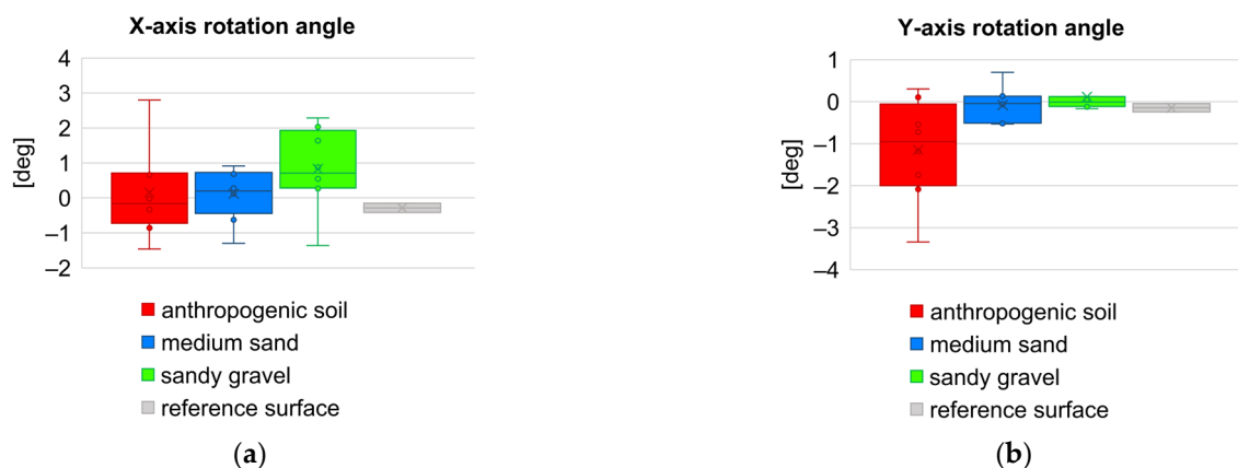
Figure 16. Box plot comparison of inclination angles of the wall surface: (a) deviation from verticality; (b) deviations from straightness (along the diaphragm wall).
