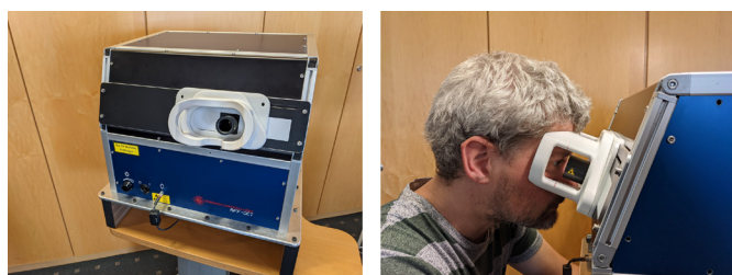
Figure 1 The Self-Examination Low-Cost Full-Field Optical Coherence Tomography prototype. Left: the three-dimensional-printed headrest is mounted on horizontal rails and can be slid freely so that both eyes can be measured. Right: author MMo demonstrates the patient's head position during measurement.
