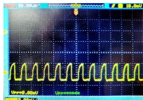
Figure 13. Optically measured pulse response of the proposed optoelectronic Rx IC.
