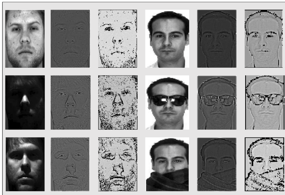
Figure 2. Photometrically distorted images from Yale database (first column) and their Self Quotient Images (SQI) counterparts before (second column) and after thresholding (third column). Images with occluded areas from Yale database (fourth column) and their SQI counterparts before (fifth column) and after thresholding (sixth column).
