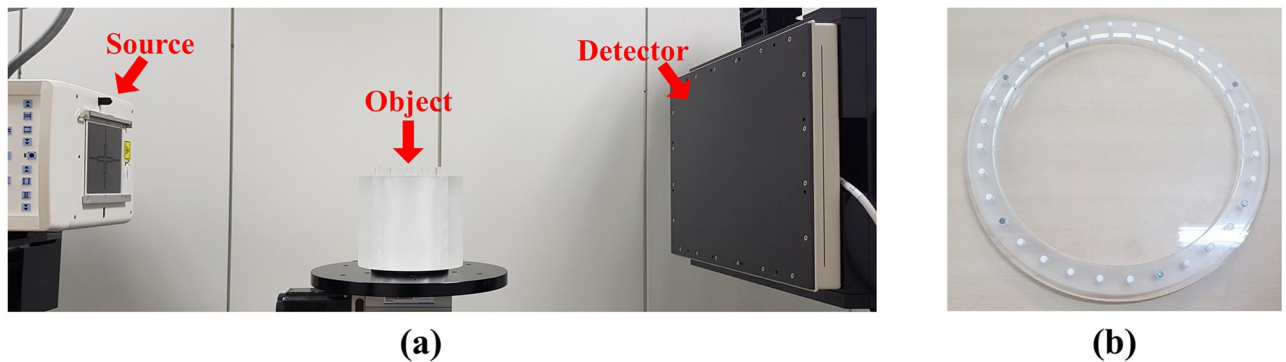
Fig 5. Experimental setup. (a) Experimental benchtop system and (b) semi-top view of the disk phantom.
