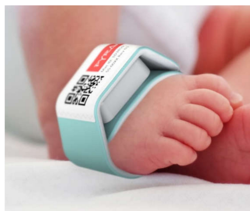
Figure 1. Boppli™ device to monitor the blood pressure of infants in critical care.
