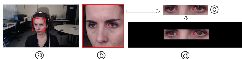
Figure 3. Image preprocessing used in the real environment experiments. The images (a) are rotated (b) so that the eyes are in the same line and cropped to the bounding box (c), which contains as meaningful information as possible. Then, a padding process (d) assures that all images have the same size before feeding them to the network. Images from the I2Head database [32].
