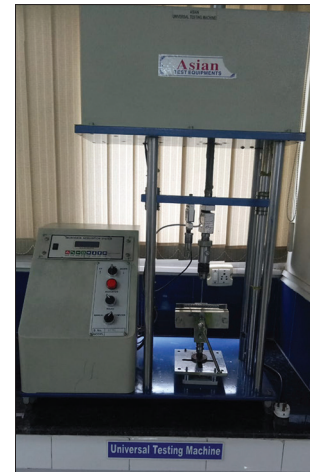
Figure 2: Diametral tensile strength calculation with Universal Testing Machine
