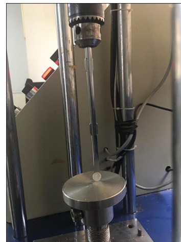
Figure 5: Close-up view of specimen in place while testing diametral tensile strength
