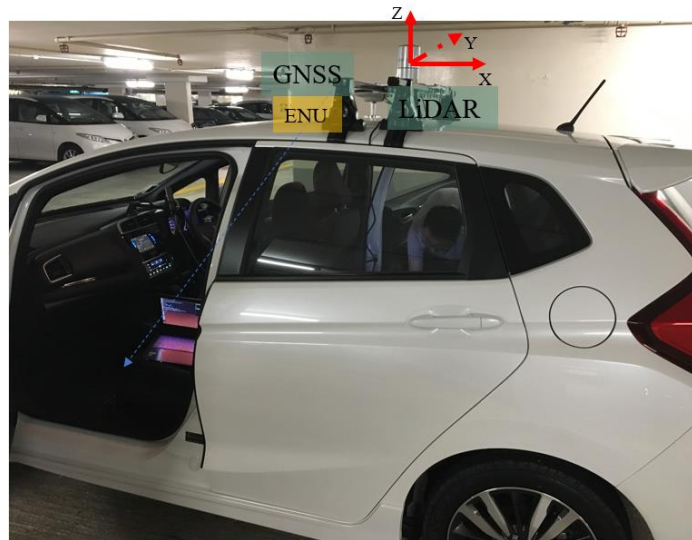
Figure 5. Sensors setup of the vehicle: 3D LiDAR sensor is installed on the top of the vehicle. GNSS RTK/INS integrated navigation system is installed on the top of the vehicle next to 3D LiDAR. The GNSS RTK/INS in ENU coordinate system is used to provide the ground truth of vehicle's position.
