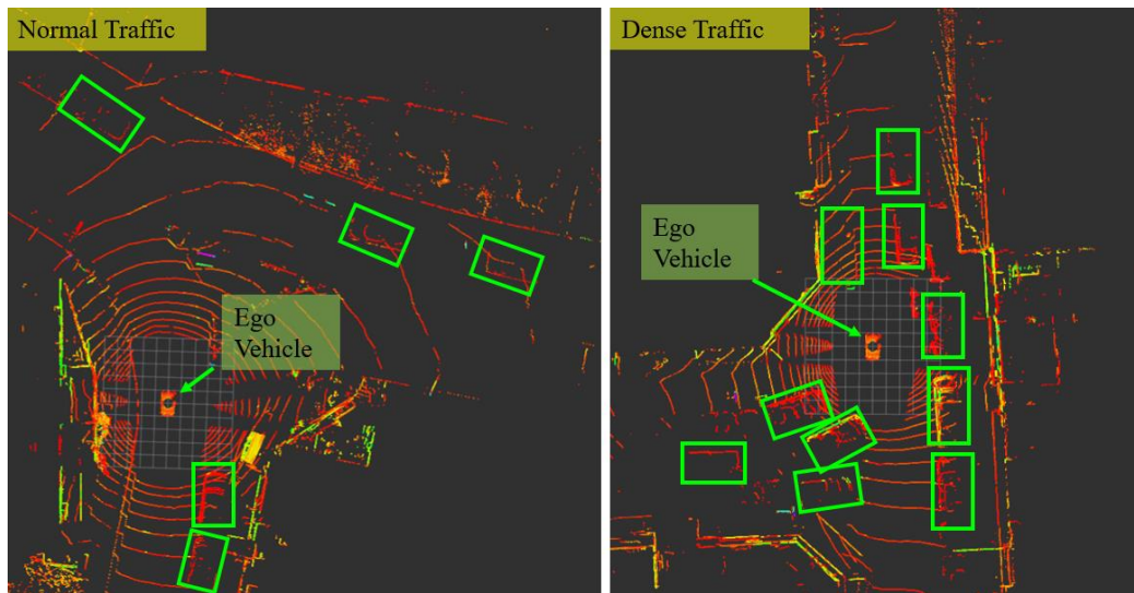
Figure 4. Scenarios with different traffic conditions. The green boxes indicate the surrounding dynamic vehicles. The left figure shows the scenario with normal traffic and right figure with dense traffic.
