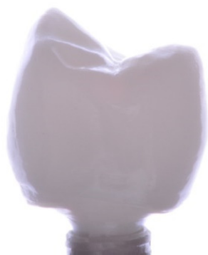
Figure 4. Stereolithography (SLA) additive manufacturing (AM) of implant supported zirconia crown after cementation.
