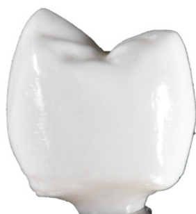
Figure 3. Stereolithography (SLA) additive manufacturing (AM) zirconia crown with buccal marginal defects.
