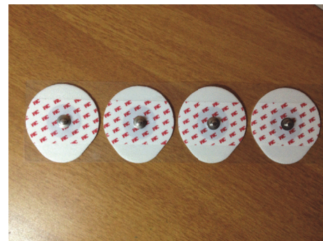
FIGURE 2: Disposal Ag/AgCl electrodes.
