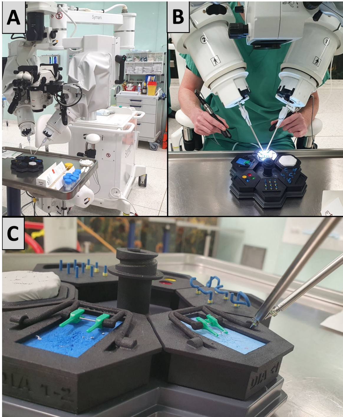
Figure 1. (A) The experimental setup using the Symani surgical system and a conventional operating microscope. (B) A robot-assisted anastomosis is performed; the robotic instruments are controlled by the participant holding the two forceps-like controllers. (C) Close-up of the robotic instruments and the vascular clamps holding an artificial vessel after completion of an anastomosis.
