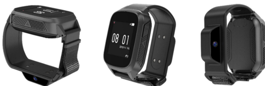
Figure 4. Camera module embedded in smartwatch for medication behavior monitoring.
