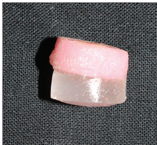
Figure 5: Finished acrylic-soft liner sample
