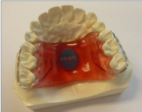
Figure 1 The SmartByte™ System. The system includes a device made of biocompatible materials that are moulded to fit an individual's palatal contour; soft edges facilitate a comfortable fit. A small, proprietary sensor is embedded within the device to precisely measure the times, frequency and duration of device use at 5-min intervals.
