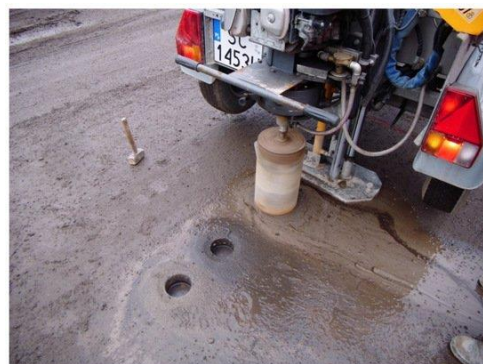
Figure 4. Pull-out test on asphalt pavement with RA.
