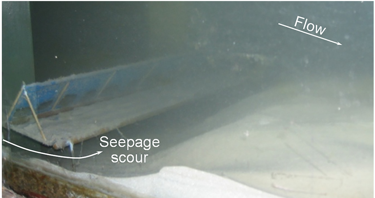
Fig 5. Seepage scour under the GMSC after 38 hours of flow by Xie et al. [24].
