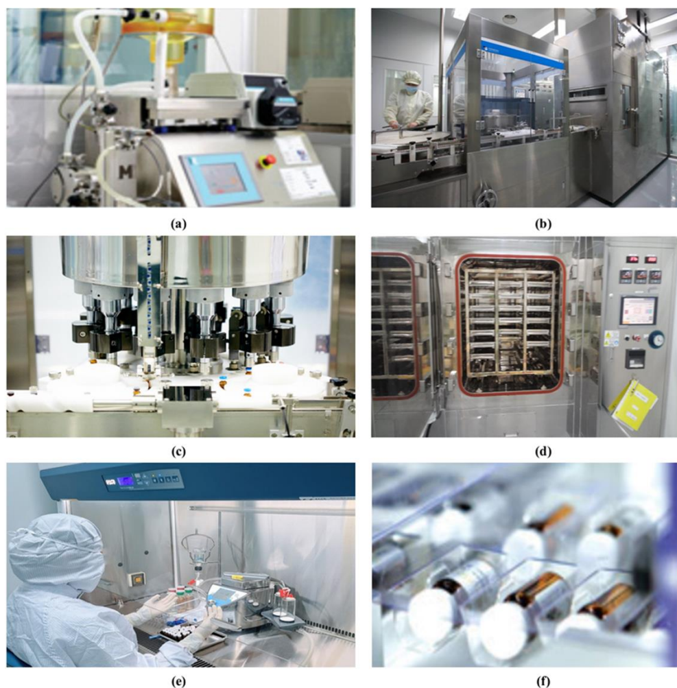
Figure 2. Preparation process of animal venom pharmacopuncture. Animal venom is prepared with pharmacopuncture through the following process; (a) venom is filtered for removing impurities and diluted with distilled water (b) vials are cleaned and sterilized (c) venom is filled and sealed into each vial (d) prepared pharmacopuncture is sterilized (e) quality inspections (e.g., sterility test, endotoxin test, and insoluble particulate matter test and pH test) are conducted and (f) packing pharmacopuncture for clinical use.
