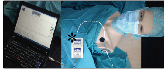
FIGURE 1: Torso phantom for simulation of a transvenous lead extraction procedure; white dashed line illustrates the course of the lead within the thorax. *Digital force gauge.
