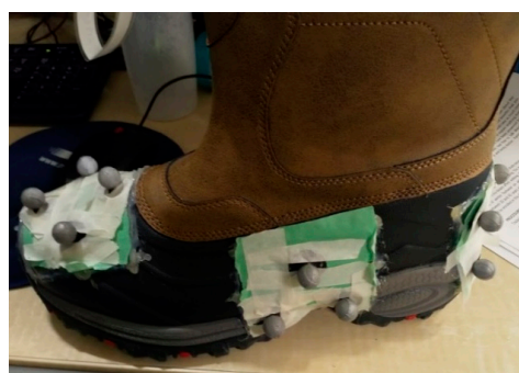
Figure 2. Reflective marker clusters were placed on the anterior, posterior and lateral aspects of each pair of test footwear.
