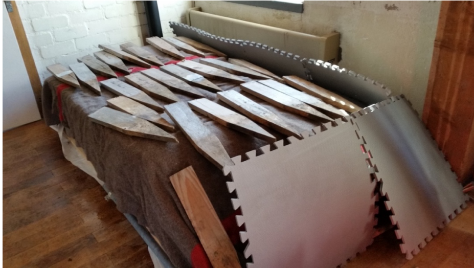
Supplementary Figure 2: Overwintering of monoliths in a cold house prior to transferring them to climate chambers. Blankets and wooden boards simulate the load of a snowpack. Digging out monoliths from snow during winter would expose them to unwanted freezing temperatures.
