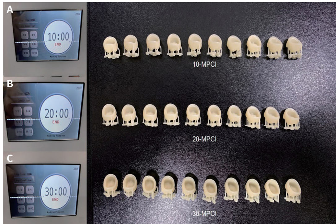
Fig. 3. Interim crowns manufactured using different post-curing processes. (A) 10-minute post-curing time (10-MPCI), (B) 20-minute post-curing time (20-MPCI), (C) 30-minute post-curing time (30-MPCI; n = 10 in each group).
