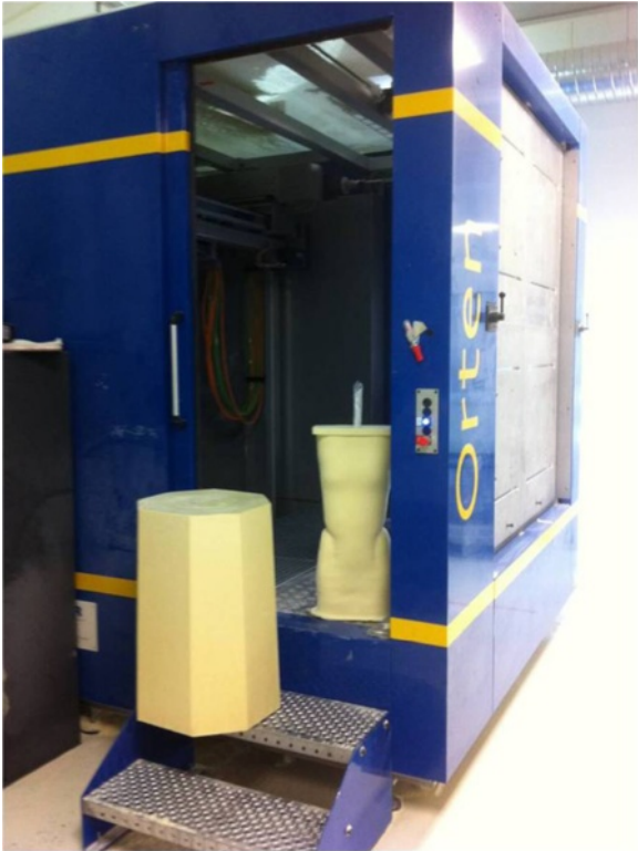
Figure 11 Milling different steps in rectifying positive.
