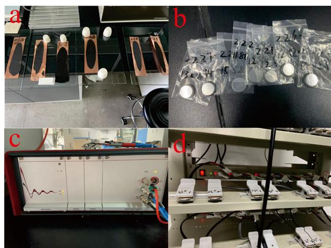
**Figure 1.** (a) Graphite mixed solution on copper sheet; (b) CR2032 button cells; (c) impedance tester; (d) electrochemical workstation.
