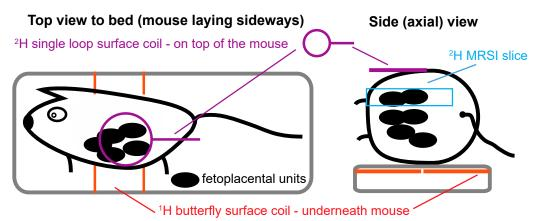
**Figure 6.** Cartoon depicting the layout used in the experiments described in this study; the <sup>1</sup>H butterfly coil is embedded in the bed itself.
