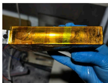
D Obvious deformation on the side of the battery
