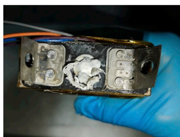
C Battery safety valve damaged
