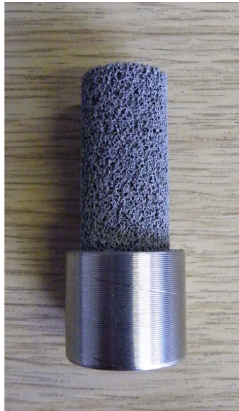
FIGURE 2. Close-up of a single test cylinder on a minisubstrate.
