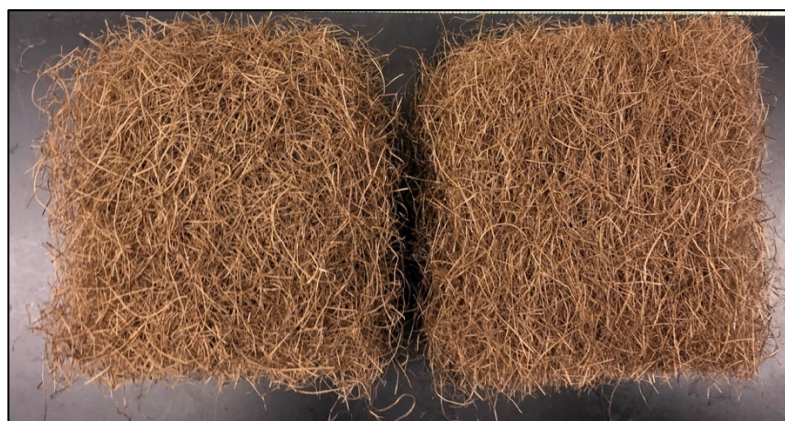
Figure 2. Example of fiber mats prepared from (left) OB fibers and (right) whole fibers of grape cane fibers.
